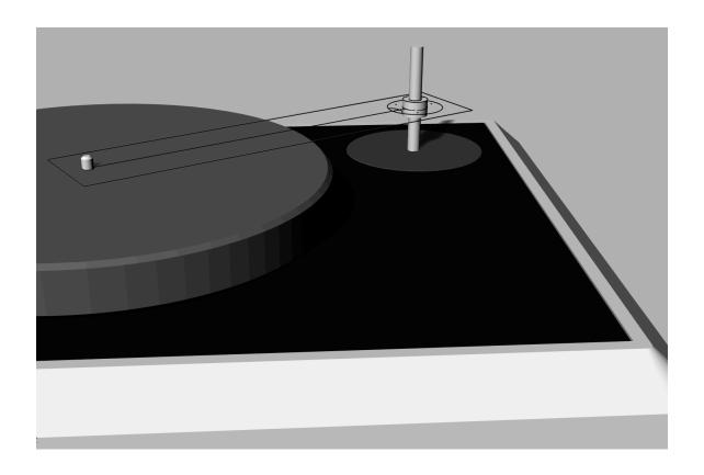
Next, take the template and insert the VTA mounting part into the 24mm hole. Mark the three holes and drill holes with a 3.5mm drill.
